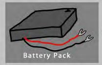
We use a 4 AA Battery Pack with attached terminals, however Squishy Circuits can be used with other battery packs.
